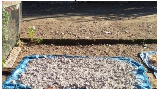
Figure 8. Drying process for marble waste
