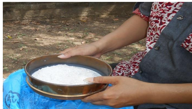
Figure 10. Marble waste sieving process
