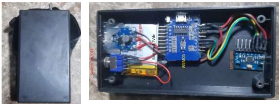
Figure 4. Android-Based Calorie Counting Device with Accelerometer Sensor
