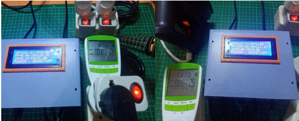
Figure 11. Voltage Detection Tests using Soldering Iron and Electric Iron
