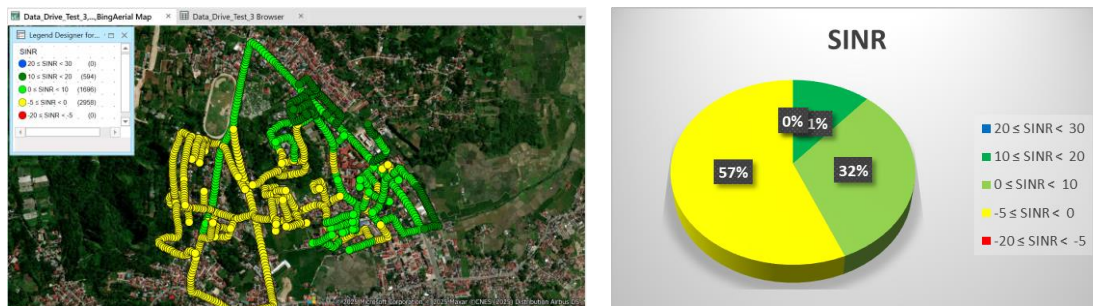
Figure 5. SINR coverage area and SINR diagram
